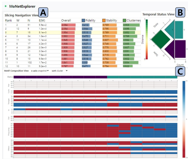
Fig. 8. Workflow of P2 validating the window size of 7 months. (A) Select the window size. (B) Observe detected snapshot states and their distances. Two different snapshot states are detected. (C) Observe motif compositions of snapshot states. In this case, the two states are well-distinguishable with their difference in ping-pong and triangle-type motifs.
