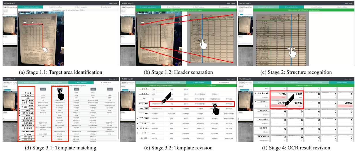
Figure 2: Figures describing stages of the mixed-initiative pipeline. (a) Users can select the target image at the left component. The selected image appears at the right component. With a mouse click, users can draw a quadrangle surrounding the target area. (b) Users can add one horizontal line and one vertical line respectively to distinguish header cells from others. (c) Based on lines that the automated model predicted, users can modify each line. Also, users can select multiple lines with drag & drop interaction and manipulate them simultaneously. (d) The automated model extracts data from the divided cells with the OCR module. With Case-based reasoning, five candidates of the template are given. Users can choose the most similar candidate among the candidates. (e) After selecting the candidate template, users can modify minor errors of header values. (f) Finally, users modify money amount values and submit the result.
